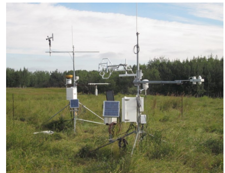
Research instruments for measuring precipitation and plant water use at Spyhill site near Calgary.
