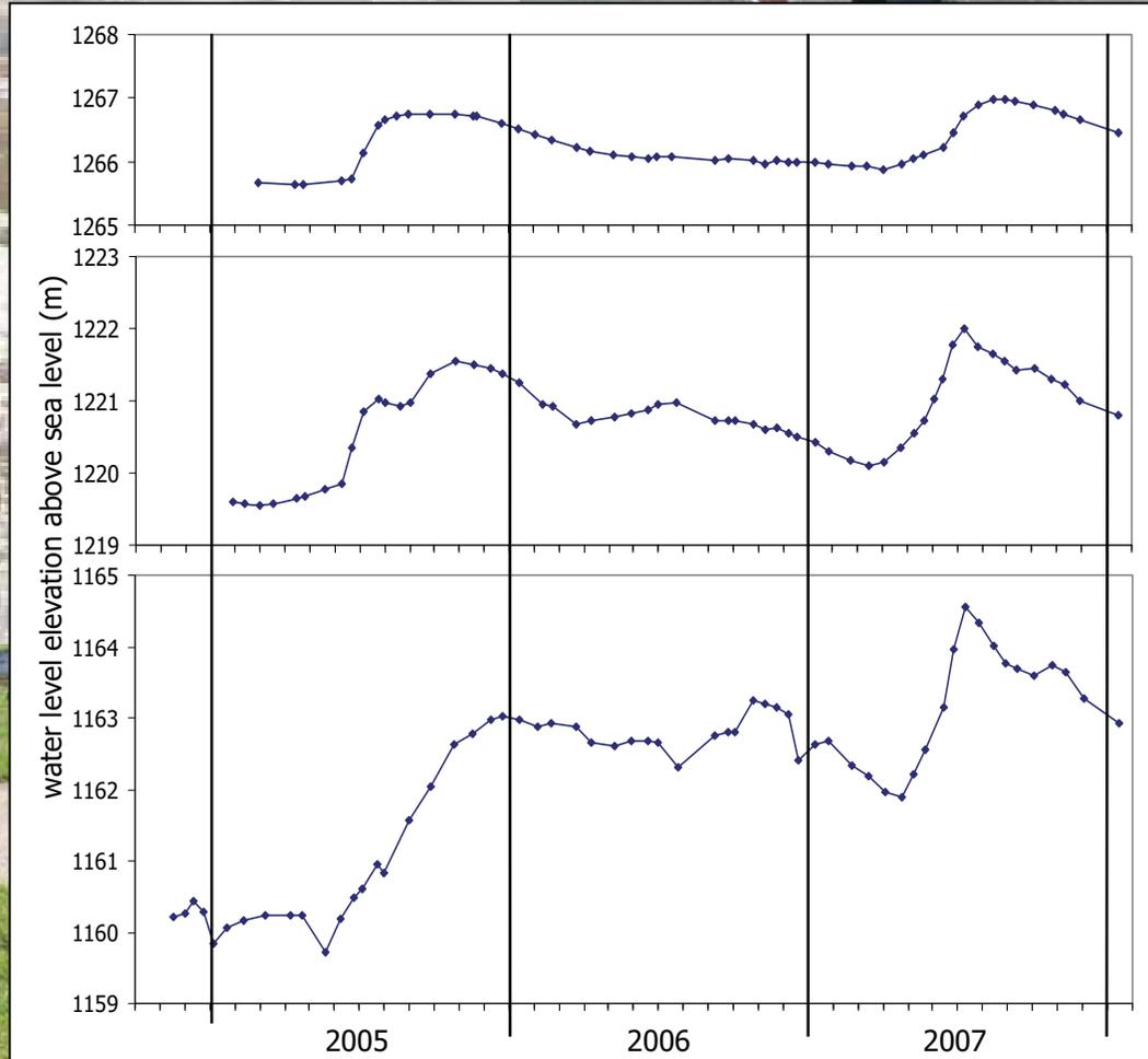
The range of water levels measured in 80% of the wells in the Monitoring Network are within three meters of the static water level reported in the drilling record, regardless of the age of the well. This means that drilling records are still a reliable indicator of water level, and that groundwater levels have not changed significantly from when the wells were drilled.
