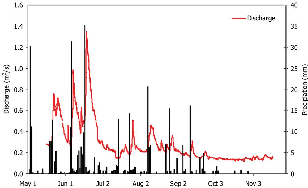
The discharge graph of West Nose Creek, as measured at the bridge on Symon's Valley Road (Hwy 772). Precipitation as measured in the watershed is in black. Water levels and discharge rapidly increase during a rain storm, and slowly decrease after.
